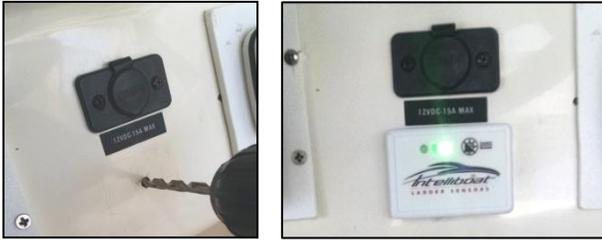
2. Use an alcohol swab to clean the area before drilling and installing the control module.
